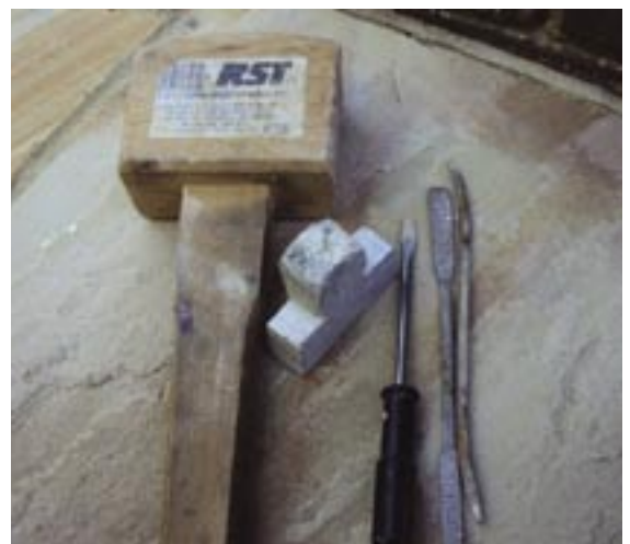
Some of Suviwan's carving tools: a mallet, screwdriver, files and riffler tools
